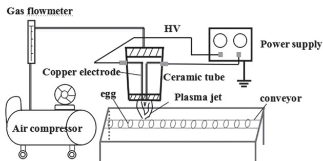
Fig. 1. Equipment schematic diagram of sample handling and packaging.
